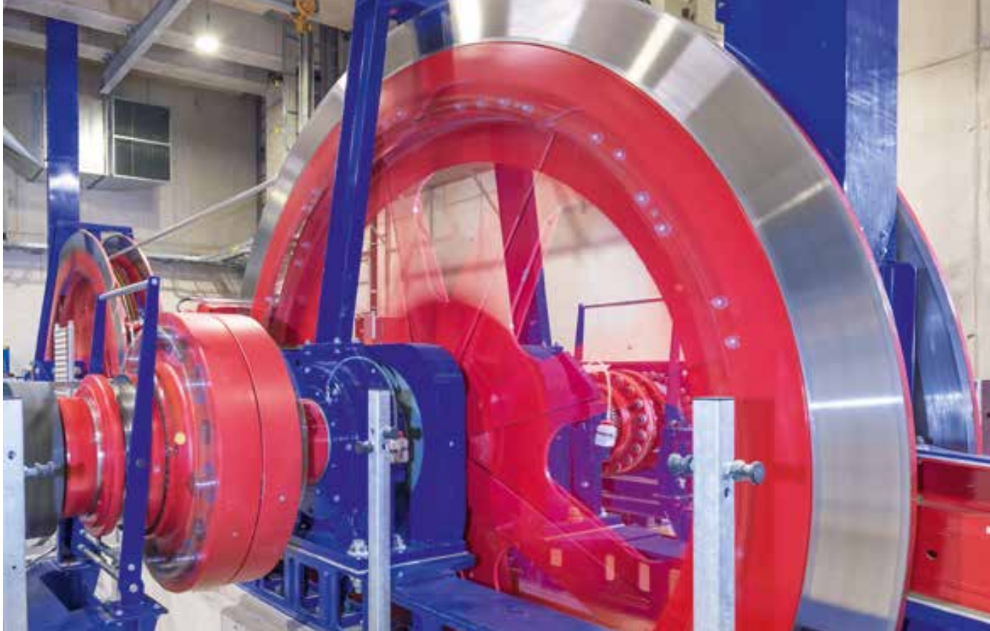
BECORIT develops, manufactures, and inspects traction sheave linings for rail vehicles. © DOPPELMAYR
