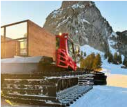
Rubber tracks prevent damage caused by traditional aluminum or steel tracks.
