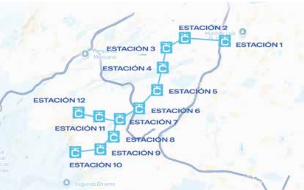
The 15.2-kilometer-long cable car line comprises 12 stations, 462 10-person cabins, and 114 towers. The connection to the Mixcoac metro station (Lines 7 and 12) strengthens integrated mobility in the west of Mexico City. The time savings amount to more than 50 percent.
