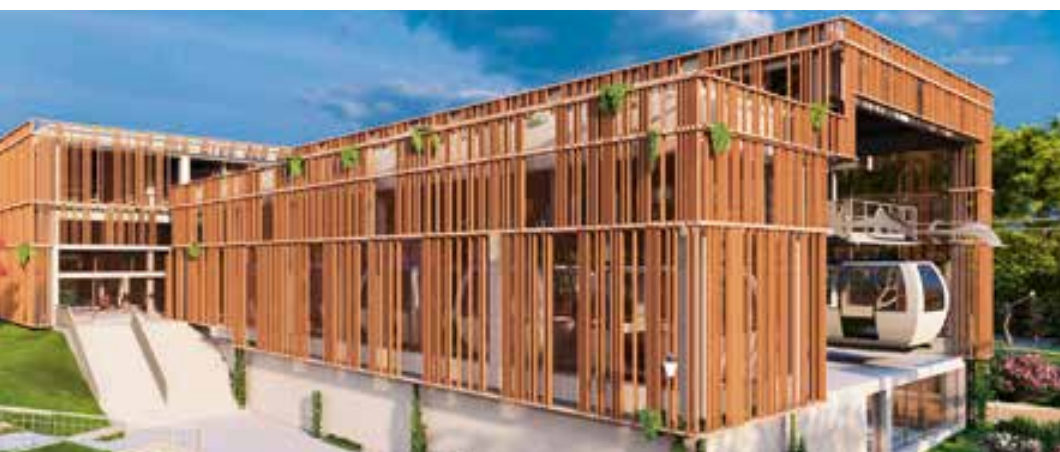
The stations will be almost completely rebuilt and made fully accessible. The facades are planned to be clad in wood, so that they blend better into the surrounding landscape.
