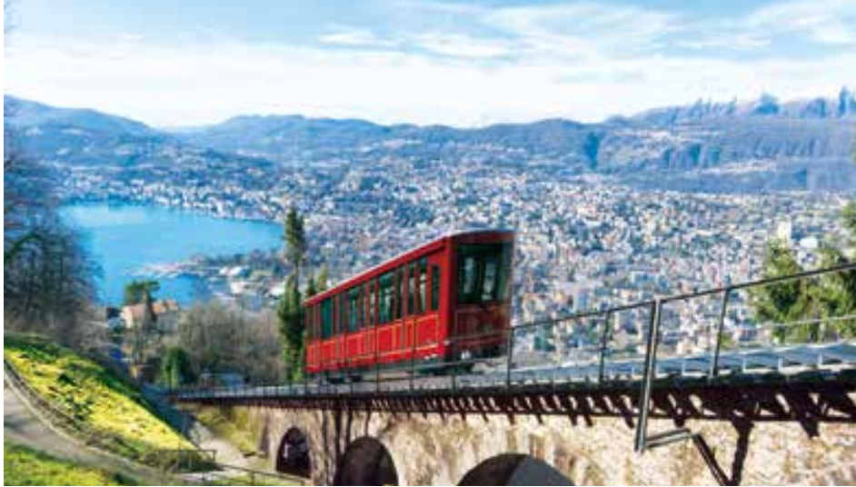
The Monte Brè funicular in Lugano features two retro-style cars designed for passengers with reduced mobility, accommodating up to 70 people. © Garaventa AG
