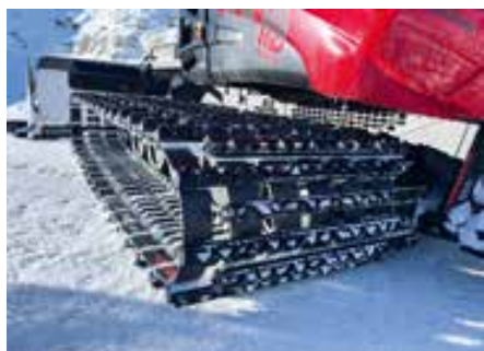
XTrack 1,420 mm is the all-season chain solution for medium alpine applications with optional spike ice grippers for icier conditions.
