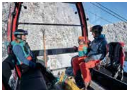
The STELLA cabin type was developed specifically for the TRI-Line and holds 18 people.
