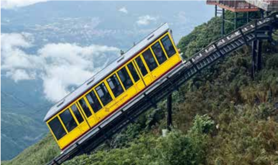
The Fansipan Coaster is characterised by its exceptional route profile with sharply varying gradients. The route rises significantly towards the end. © Garaventa
