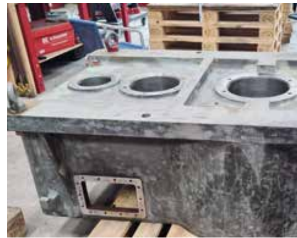
The sandblasted gearbox is inspected for material cracks by Kissling AG using UT/MT (ultrasonic / magnetic particle testing).
