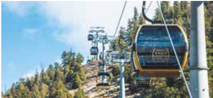
The 10-MGD Mighty Argo Cable Car spans a length of 1,681 meters, climbs 396 vertical meters in ten minutes, and carries up to 1,300 passengers per hour utilizing 22 cabins. © Mighty Argo Cable Car
