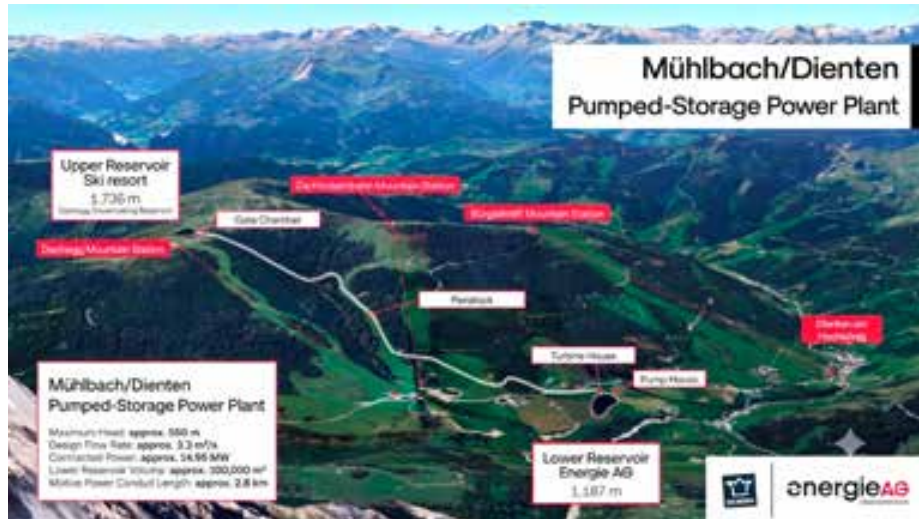
The visualization of the pumped-storage power plant in Mühlbach/Dienten. © Energie AG
