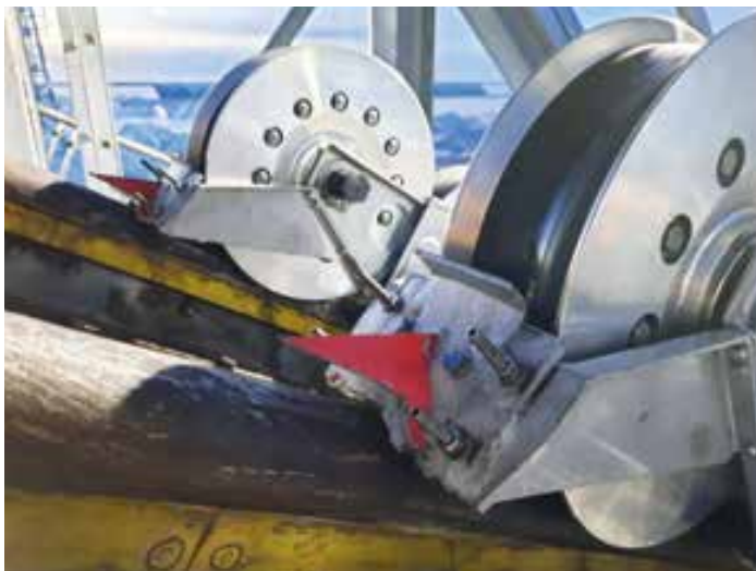
Ice scraper (left) and white hard plastic roller on the drive system of the Zugspitze cable car.
