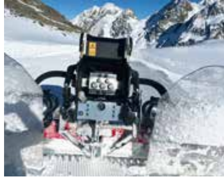
The tiller can be uncoupled in seconds with the KFX. © KÄSSBOHRER
