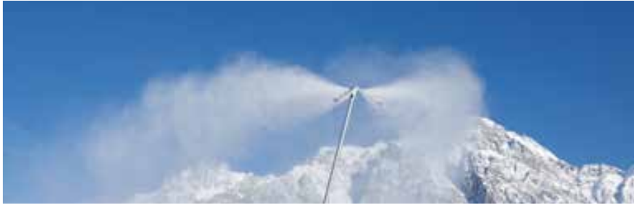
SnoTek V1 6D MEDUSA lance head as a retrofit replacement on an existing Sufag Taurus system.
