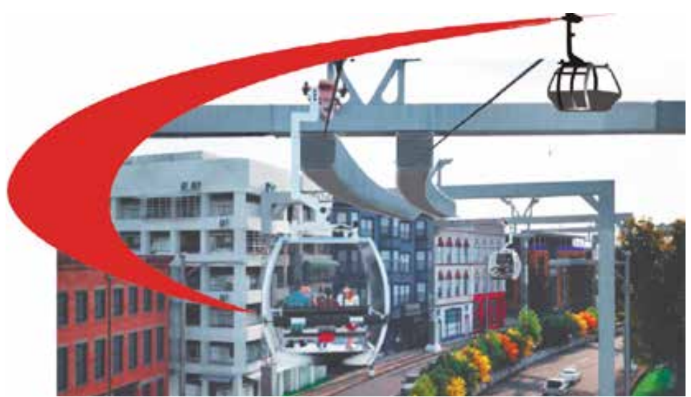
CURVO ropeway incorporates the patented vertical grip technology and the angular module to negotiate bends at line speed without detachment.
