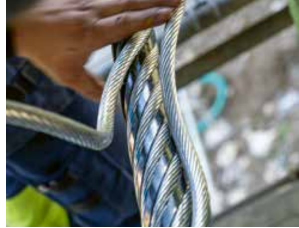
With TRUsplice ES , the high quality of the splice on the PERFORMA rope is maintained. © FATZER
