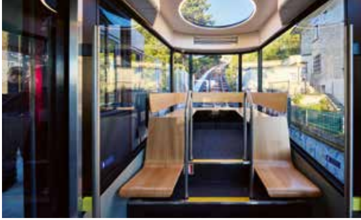
A round skylight with a lighting ring brings additional daylight into the cabin, especially over the raised seating area.
