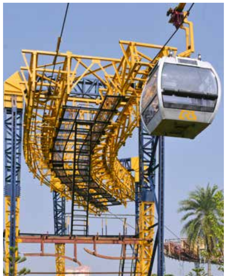
CURVO is a Non-Linear Monocable Continuous Gondola system.
