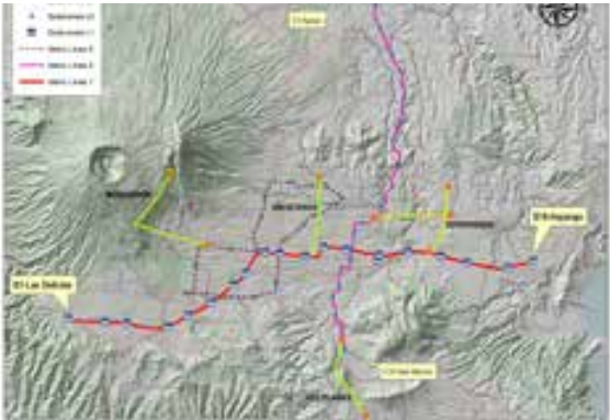
Master plan with four cable car lines (in green): one goes to the volcano (Boquerón), one runs through the city center (Mejicanos), one heads south (Los Planes) and one will serve the east district (Soyapango).
